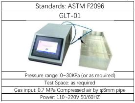
**Micro Leak Tester** is based on vacuum decay method, and is a non-destructive way for leak testing of rigid and semi-rigid non-lidded trays; trays or cups sealed with porous barrier lidding materials; rigid, nonporous packages; and flexible, nonporous packages.
